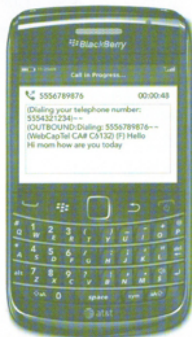
The Hamilton CapTel mobile phone translates speech into text. Photo courtesy of Oaktree Products.
